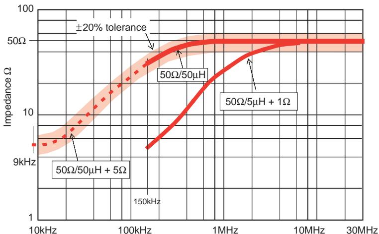
**Figure 4** - Impedance curve of CISPR AMN / LISN
