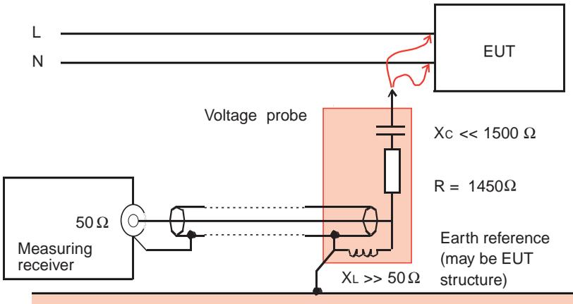
Figure 7 - Use of the voltage probe
