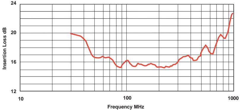
Figure 9 - Typical clamp calibration curve
