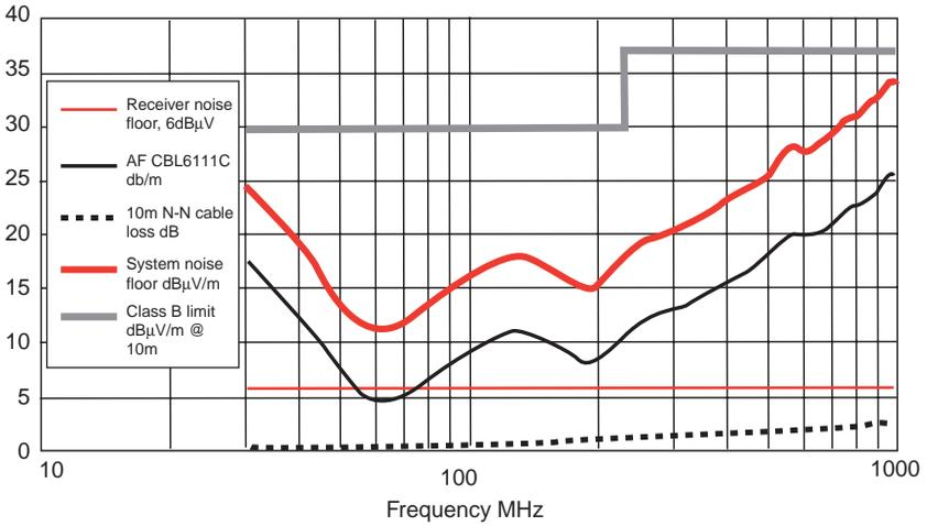
Figure 14 - Typical calibration factors of Schaffner-Chase antennas
