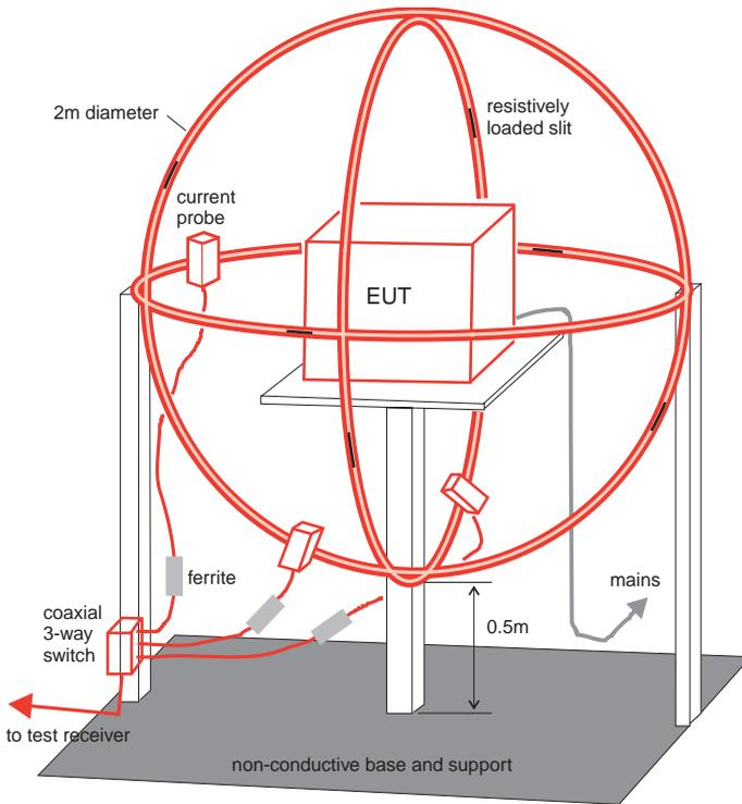
Figure 19 - Large loop antenna setup
