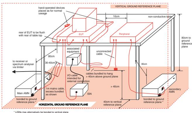
Figure 5 - Conducted emissions test layout
