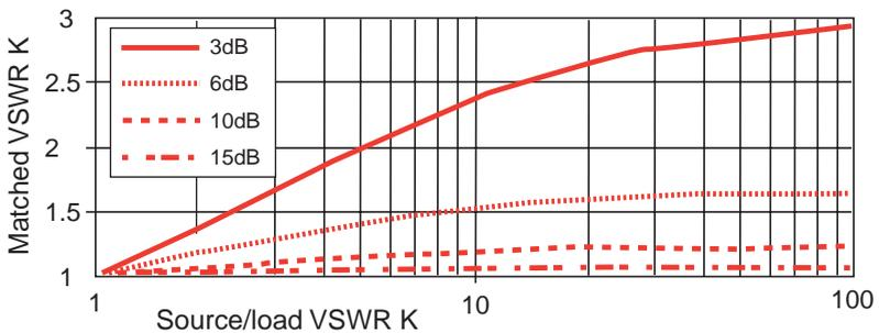
Figure 23 - Improvement of matching with an attenuator
