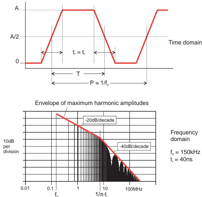
Figure 24 - Trapezoidal waveform and harmonic envelope
