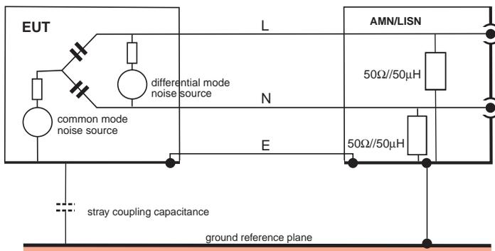
Figure 6 - General conducted emissions equivalent circuit
