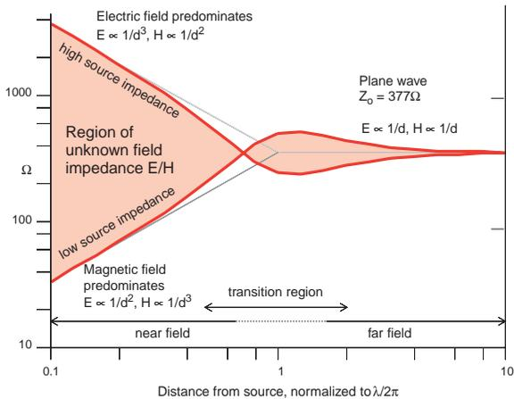
Figure 21 - The wave impedance
