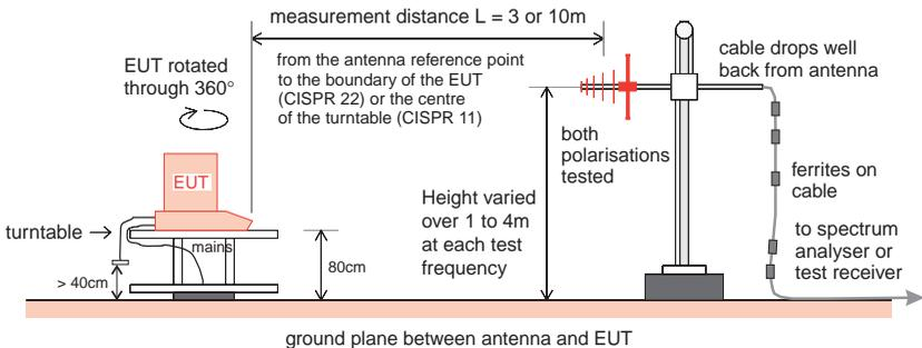
**Figure 11** - Setup on the open area test site
