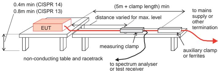
Figure 10 - Test setup for absorbing clamp
