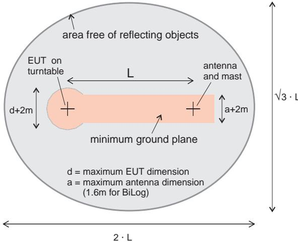
Figure 12 - Plan view of the minimum CISPR OATS
