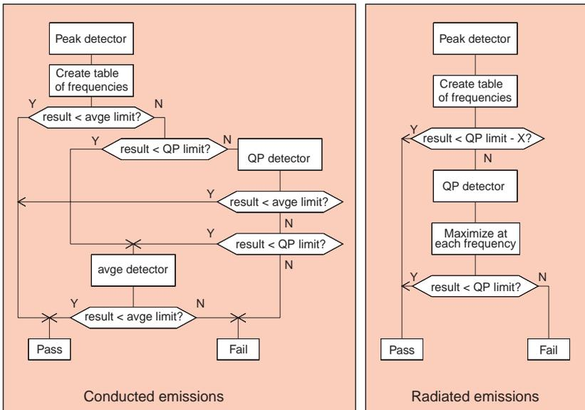
Figure 2 - Flow chart for use of detectors
