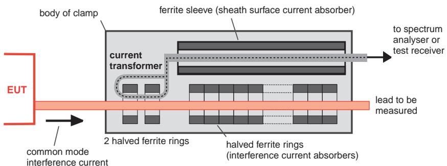
Figure 8 - Construction of the absorbing clamp
