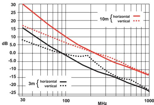
Figure 16 - Theoretical NSA for broadband antenna geometries
