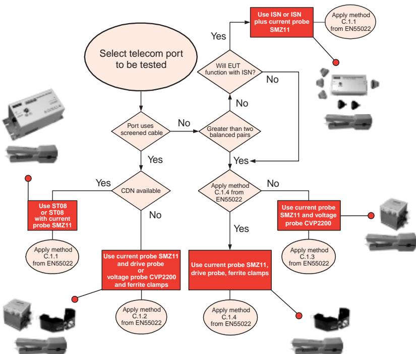
Flowchart to determine test method for telecommunications ports
