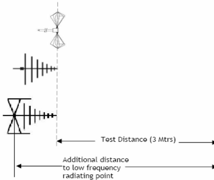
Figure 5 - Definition of antenna to EUT distance
