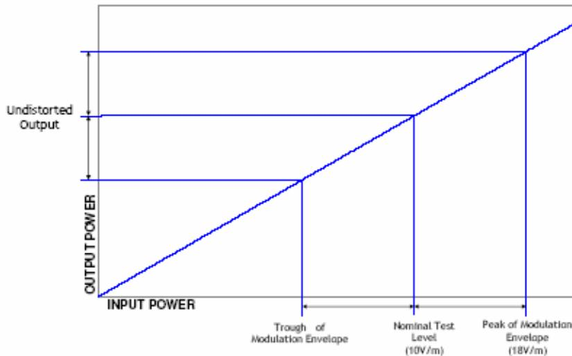
Figure 3 - Amplifier operated in linear range
