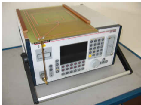
Fig. 2a Test device for immunity tests
